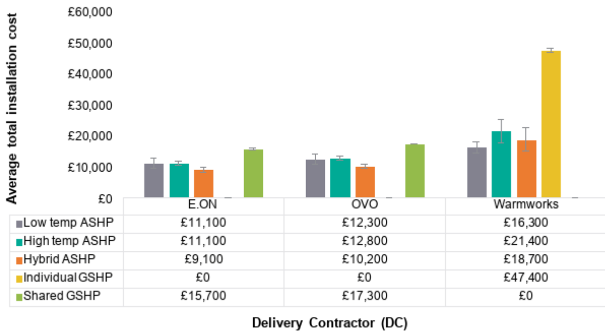
Figure 26 Average total costs of heat pump installations by DC, including additional measures
